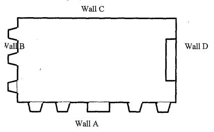
Evaluation of Exterior: The parapets on the A, B, C and D side present an imminent hazard and must be removed as specified below. All falling hazards endangering the public must be removed. Any unsupported portions of flooring and walls must be removed as described below.
