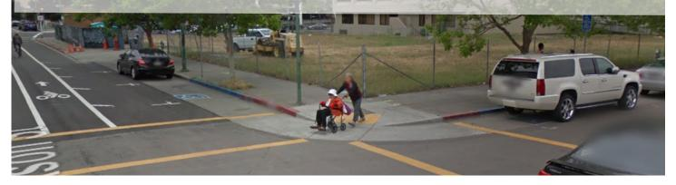
Missing pedestrian signals and push buttons. Intersections do not provide pedestrian signals or a pedestrian phase. Existing traffic cabinet with not service cabinet. Cabinets require upgrade to provide pedestrian countdown signals and accessible pedestrian signals.
