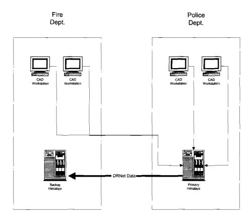
Single Box Configuration - Showing Normal Operation System Diagram 1
